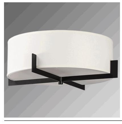
18" Ceiling Fixture with Matte Black Accents, three GU24 sockets, direct wired, with 15.5x15.5x4 Cream Linen Hardback shade with single fold trim and frosted white acrylic bottom diffuser. Recommend three 1100 lumen LED bulbs with GU24 base. 18"W, 6"H
